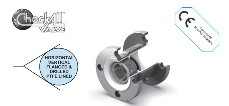
The Check-All® Flanged & Drilled — Fluoropolymer (PTFE) Lined (HT) check valve is a one piece body with ANSI/ASME B16.5 Class 150 flanged ends. The valve has a solid one piece PTFE liner which covers the flange faces out to the raised face diameter. All wetted surfaces are fluoropolymer (PTFE/FEP/PFA) including the FEP encapsulated stainless steel spring.
