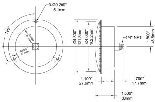
Front flange is a standard integral part of the 3.5" back connection case
